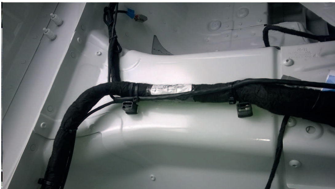
Figure 5.9: ABS loom on top of center tunnel
