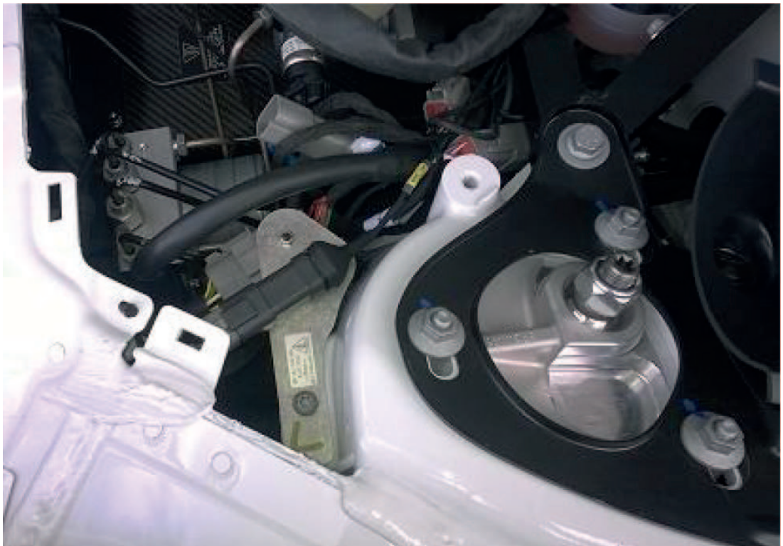
Figure 4.5: Wiring loom position at ABS exit
