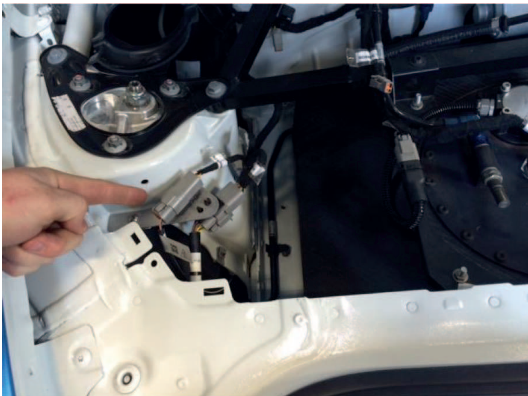
Figure 4.7: Wheel speed sensor FR connector without ABS
