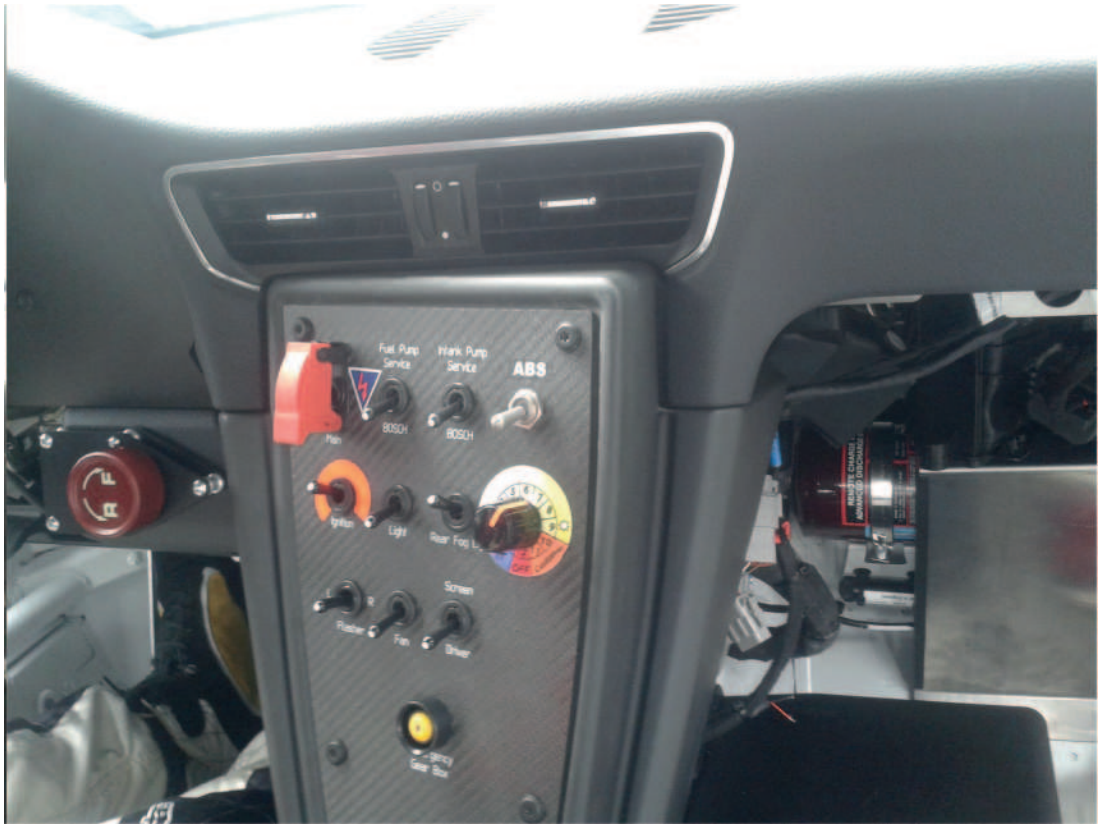
Figure 5.5: ABS On/Off and ABS 12-position switch
