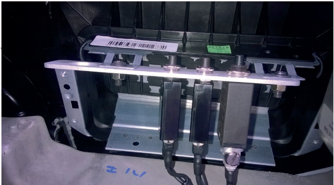
Figure 5.3: Bracket with fuses and hole for ABS diagnostic plug on the Cup Gen 1
