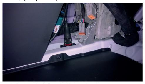
Fig. 19: Wheelspeed signal splitter with wiring loom plugged in
