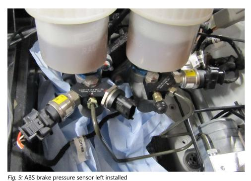
This is the last step of the installation of the brake hydraulics.
