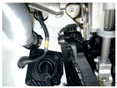
Fig. 24: ABS loom runs from connection point upwards
