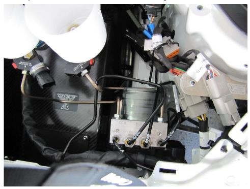
Fig. 8: Brake pipes connected
