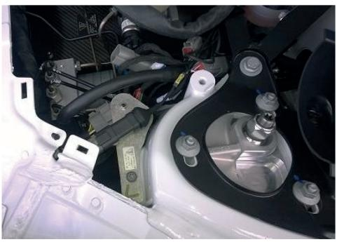
Fig. 14: Wiring loom position at ABS exit
