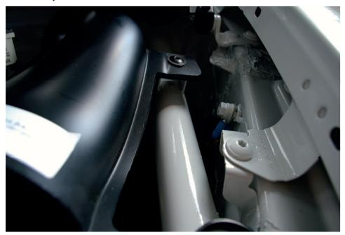
Fig. 13: Connection of ground cable
