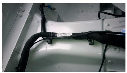
Fig. 26: ABS loom on top of center tunnel
