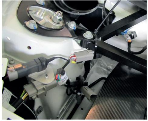
Fig. 17: ABS loom connected
