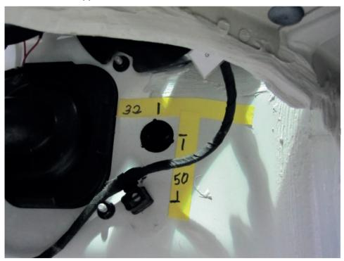
Fig. 10: Position of hole in bulkhead
