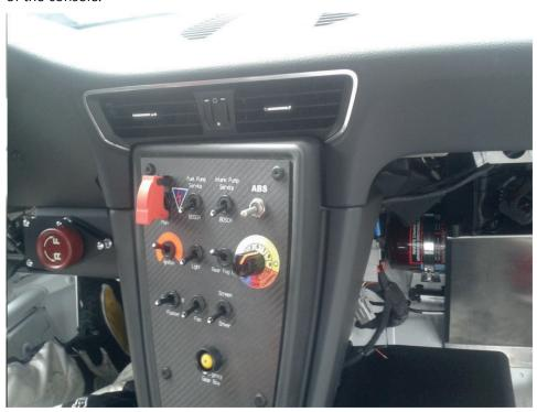
Fig. 22: ABS On/Off and ABS 12-position switch
