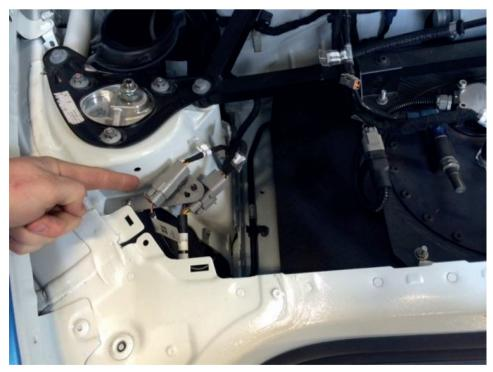
Fig. 16: Wheel speed sensor FR connector without ABS
