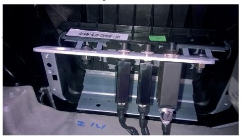
Fig. 20: Bracket with fuses and hole for ABS diagnostic plug on the Cup Gen 1
