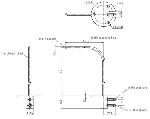
total pressure = static pressure + velocity pressure
