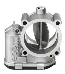
The electronic throttle body (ETB) is part of an electronic throttle control system (ETC). The ETC contains furthermore an electronic acceleration pedal or a redundant rotary potentiometer for a mechanical throttle body.
