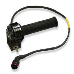
This Electronic Throttle Grip (ETG) eliminates the throttle cables connecting the throttle grip and the throttle body and replaces them with an electronic connection.
