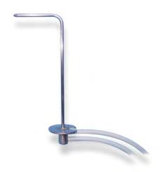
The pitot tube PT is designed to measure the vehicle speed relative to the surrounding air. Its main application is the aerodynamic car setup. The pitot static tube consists basically of two concentric tubes. The ellipsoidal nose form has a single forward facing hole for sensing total pressure and a ring of side holes for sensing the static pressure. Measuring the difference of both pressures (see Bosch different pressure sensor), the velocity related to the air can be calculated
