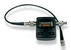
The FM 40 Tester is used to check the performance of telemetry components installed in the car which includes the FM 40 in conjunction with the RF wire and the antenna. The FM 40 tester indicates RF output power as well as defective RF wires or car antennas enabling quick detection of faulty components.
