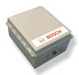
The Pit Receiver Box integrates all electronic components necessary to receive telemetry data from a car equipped with a FM 40 transmitter in one weatherproof package. Typically the receiver box is mounted on the pit roof as close as possible to the RX antenna, thus minimizing cable loss. The connection wire to the receiving PC in the garage, which can be up to 50 m long, also supplies power to the Pit Receiver Box.
