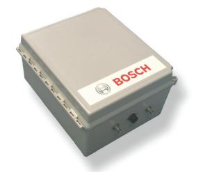
The Pit Receiver Box integrates all electronic components necessary to receive telemetry data from a car equipped with a FM 40 transmitter in one weatherproof package. Typically the receiver box is mounted on the pit roof as close as possible to the RX antenna, thus minimizing cable loss. The connection wire to the receiving PC in the garage, which can be up to 50 m long, also supplies power to the Pit Receiver Box.
