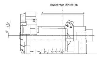
IN CASE OF MOUNTING POSITION WITH DC-MOTOR ON TOP A COMBINATION OF THE ANGLES SHOWN BELOW IS NOT ALLOWED!
