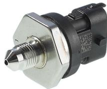
The brake pressure sensor is installed into the front axle brake circuit between the master cylinder and the hydraulic power unit. The sensor is metric thread, M10x1. Before assembly, fill the sensor with brake fluid, e.g. with a small medical syringe. So the brake system can be fully bled, the measuring hole of the brake pressure sensor should point upwards.
