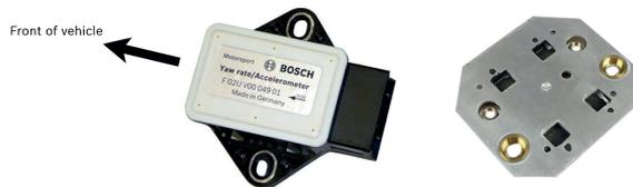
The gyro/acceleration sensor is specific to the system and should be mounted as close as possible to the center of gravity of vehicle. The sensor should be assembled with the supplied damping plate. Position the sensor so that the connector is pointing towards the rear of the vehicle.
