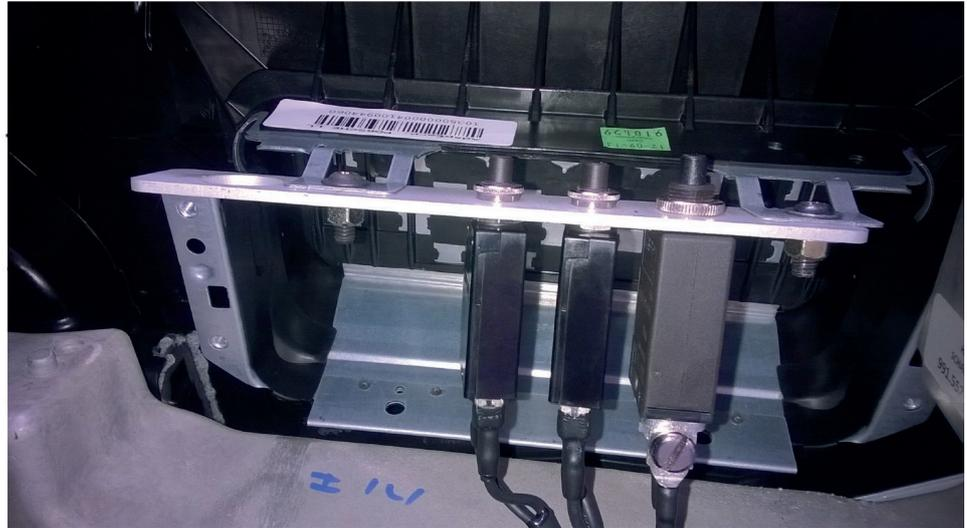
*Fig. 20:* Bracket with fuses and hole for ABS diagnostic plug on the Cup Gen 1
