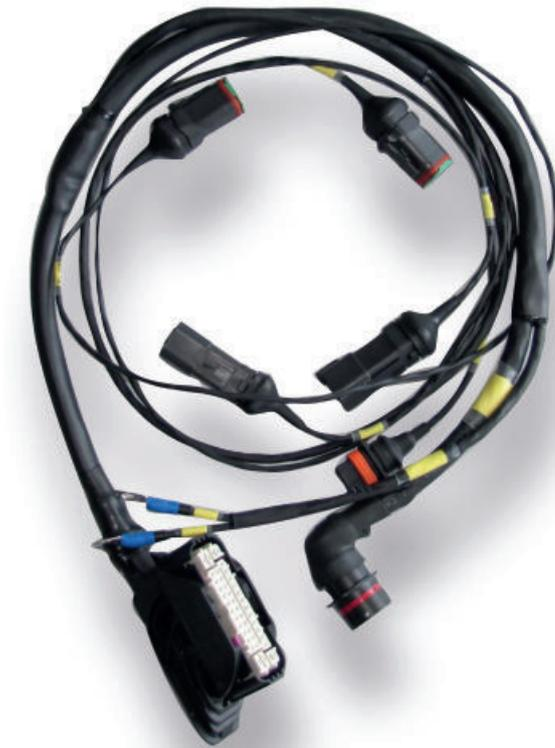
*Fig. 12:* ABS loom for front boot area
