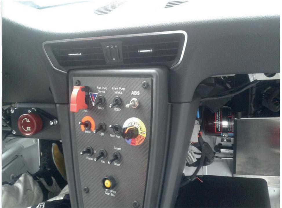
Fig. 22: ABS On/Off and ABS 12-position switch
