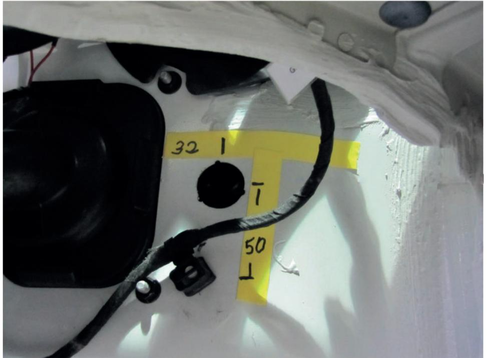
*Fig. 10:* Position of hole in bulkhead
