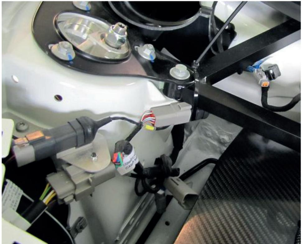
*Fig. 17:* ABS loom connected
