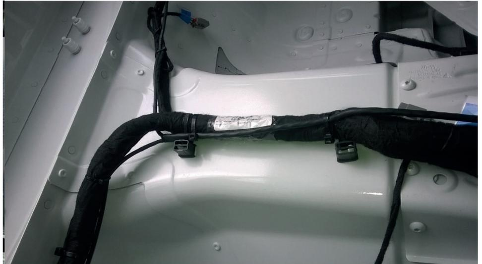
*Fig. 26: ABS loom on top of center tunnel*
