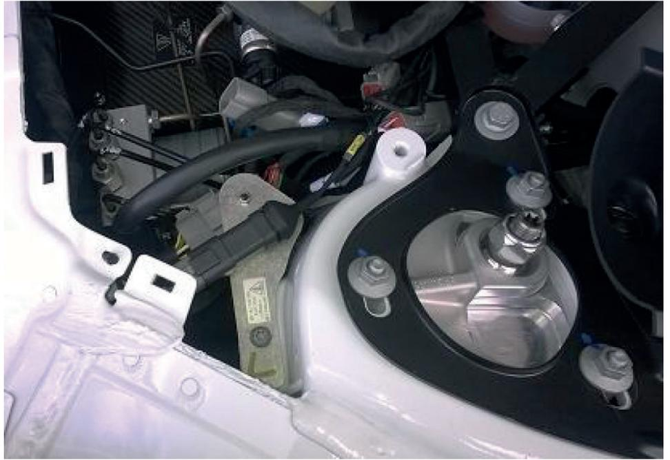
*Fig. 14: Wiring loom position at ABS exit*
