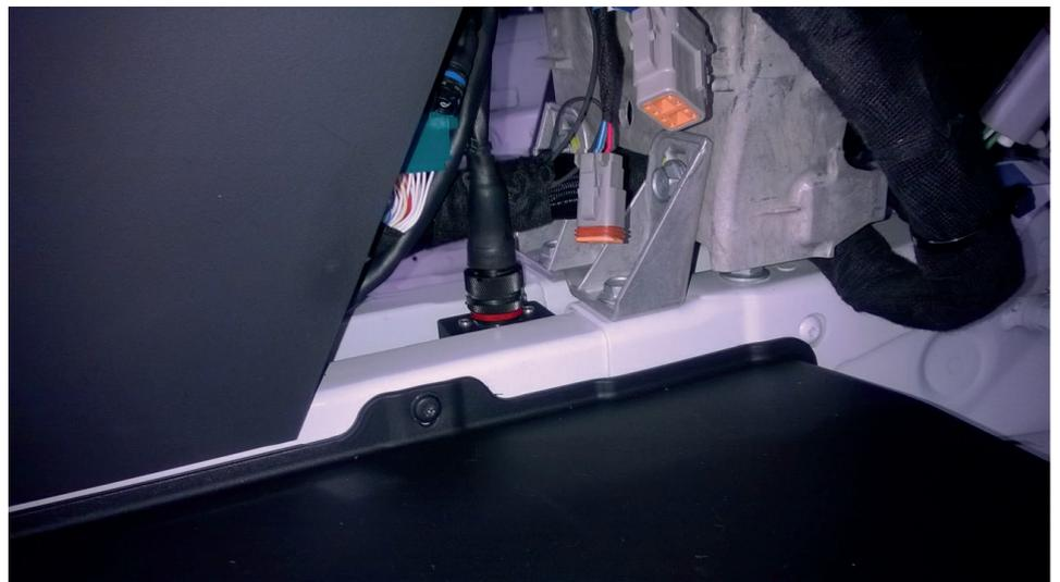
*Fig. 19:* Wheelspeed signal splitter with wiring loom plugged in
