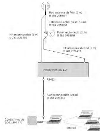
The Pit Receiver Packages 1/R contain antennas, rf wires, data wires and the controller box, i.e. everything that is required to start operation.
