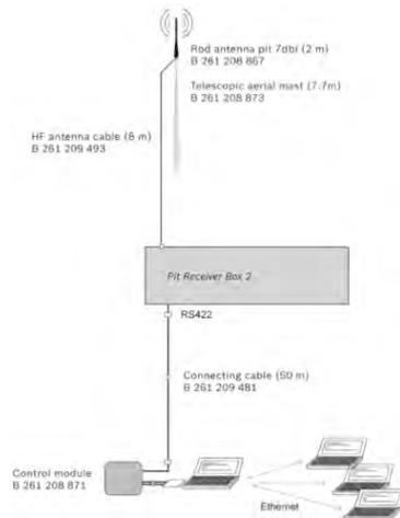
The Pit Receiver Package 2 contains antennas, rf wires, data wires and the controller box, i.e. everything that is required to start operations.
