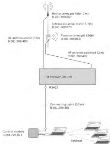
The Pit Receiver Packages 1 contain antennas, rf wires, data wires and the controller box, i.e. everything that is required to start operation.
