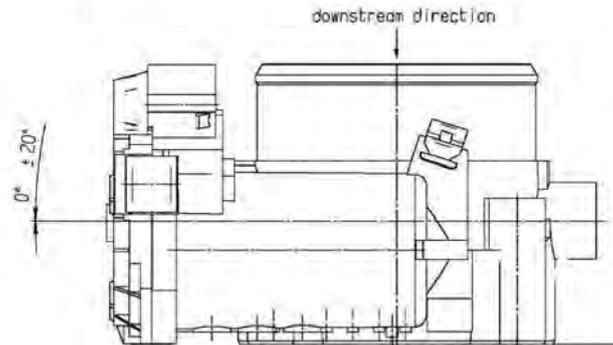
IN CASE OF MOUNTING POSITION WITH DC-MOTOR ON TOP
