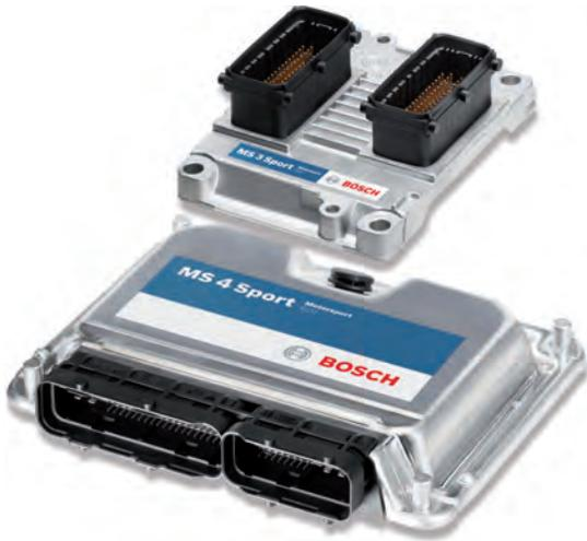
The Sport Line introduces a simple and competitive start in the world of engine control units from Bosch Motorsport. In comparison with the Performance Line ECUs from Bosch Motorsport, the Sport Line devices have an optimized function range that make the initial start-up process much simpler.
