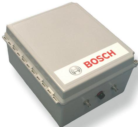
The Pit Receiver Box integrates all electronic components necessary to receive telemetry data from a car equipped with a FM 40 transmitter in one weatherproof package. Typically the receiver box is mounted on the pit roof as close as possible to the RX antenna, thus minimizing cable loss. The connection wire to the receiving PC in the garage, which can be up to 50 m long, also supplies power to the Pit Receiver Box.
