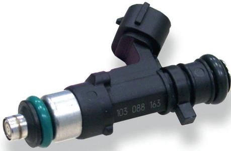
(after Methanol-operating the valves must be flushed with normal gasoline-fuel)
