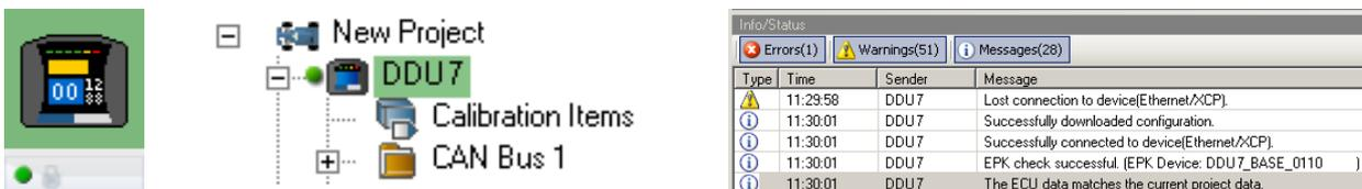
If the system's configuration in RaceCon has been changed, the dot and background becomes yellow and a configuration download is necessary.
