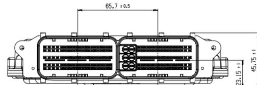
STANDING OR PERMANENTLY RUNNING WATER IS NOT PERMISSIBLE IN THE AREA OF CIRCUMFERENTIAL SEALING GROOVES, AS WELL IN THE AREA OF THE PRESSURE COMPENSATION ELEMENT. PERMITTED IMPACT OF WATER ACCORDING TO PROJECT-SPECIFIC USER MANUAL.
