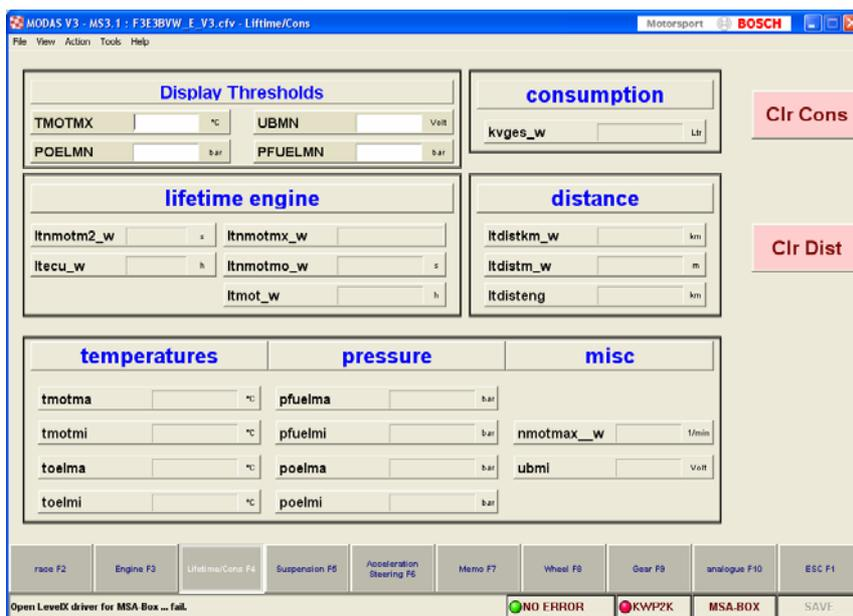
In its lifetime, the MS3.1 saves specific lifetime MIN/MAX data. This includes the operational time of the ECU (ltecu) in its life, the driven distance in km (ltdistkm\_w), the driven distance in m (ltdistm\_w), the engine operating time (ltmot\_w), the engine distance (ltdisteng), the time spent
