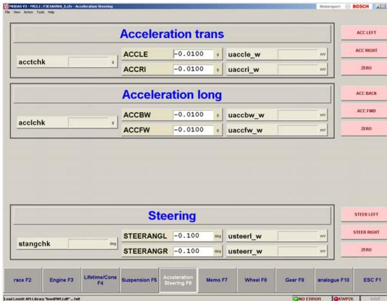
The transversal acceleration sensor can be calibrated with the “Acceleration Trans” box.
