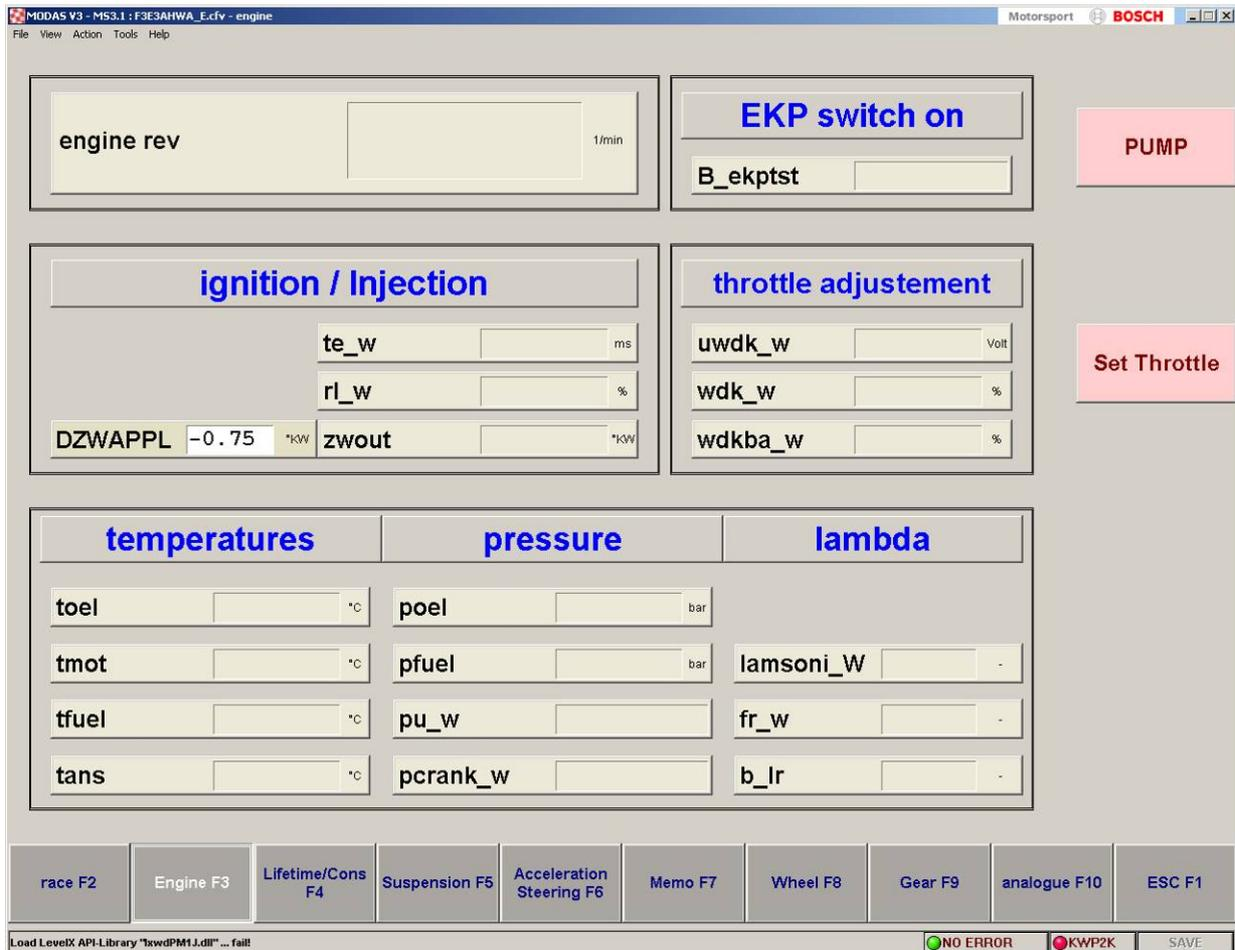
The most important engine parameters will be shown in this display. This function contains for example engine revolutions, throttle valve angle, temperatures, pressures, ignition angle, injection time.
