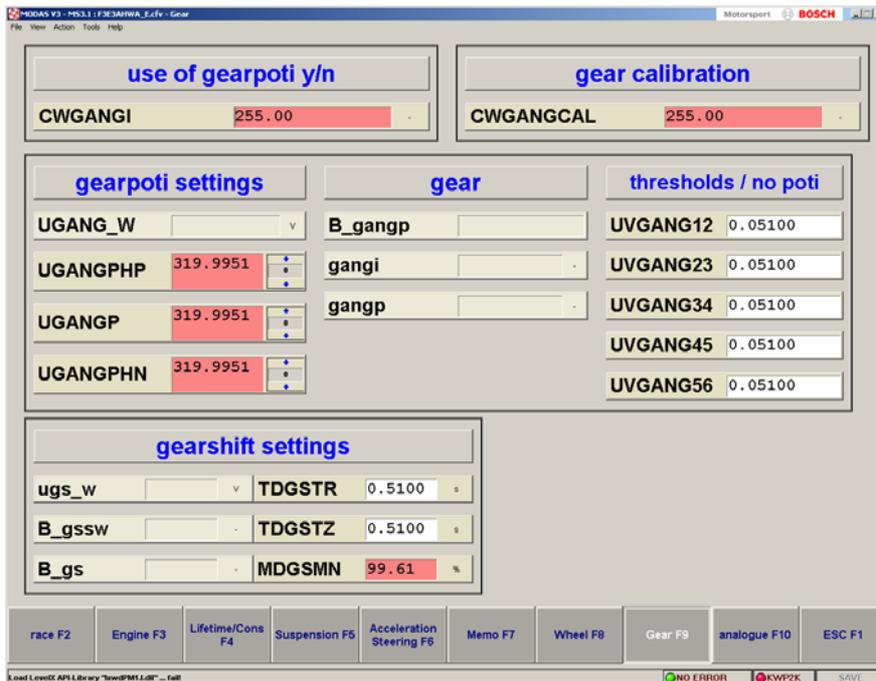
The codeword CWGANGI is used to tune whether a gear poti is attached or if the gear position is calculated via gear ratios.
