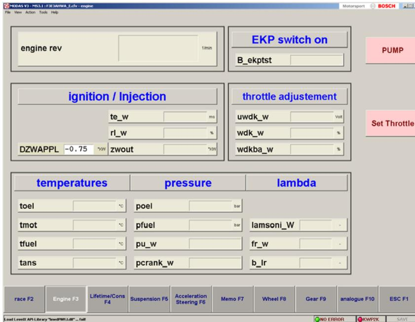
seconds when the “pump“ macro is selected. The engine must be stopped (B\_nmot = FALSE) and communication between the PC and the ECU must be active. (B\_klineok = TRUE).
