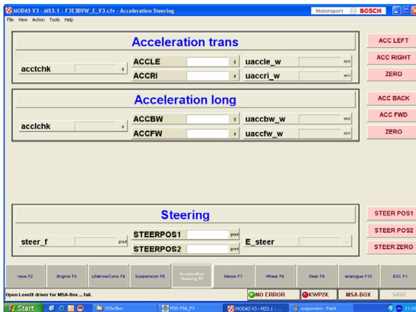
The longitudinal acceleration sensor can be calibrated with the “Acceleration Long“ box.
