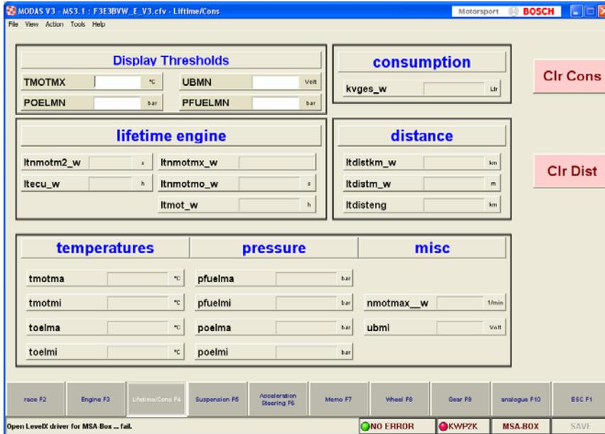
This display shows all the Min/ Max data. It includes: engine revolution (max), fuel pressure (min/ max), oil pressure (min), engine temperature (max), oil temperature (min/max), battery-voltage (min). The alarm thresholds can be set in the box “Display Thresholds”:
