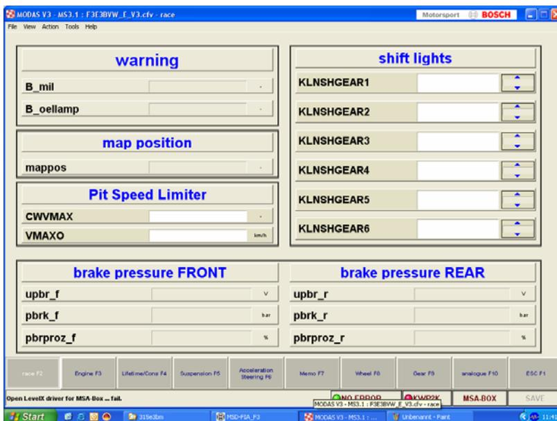
The display left, shows the map position conditions one and two, the active diagnostic LED (B\_mil = true), and the oil warning LED (B\_oellamp = true). mappos is showing the current map position.
